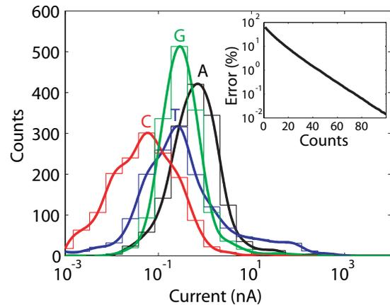
FIG. 3: Probability distributions of currents at a bias of 1 V for poly(dX)<sub>15</sub>, where X is Adenine/Thymine/Cytosine/Guanine for the black/blue/red/green curve, respectively. The thin lines show the actual current intervals used for the count, while the thick lines are an interpolation. The inset shows the exponentially decaying ratio of falsely identified bases versus number of independent counts (measurements) of the current averaged over the four bases.
