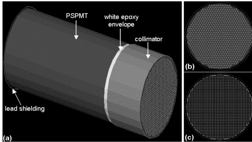
**Figure 1.** (a) Picture of the IASA scintillation camera simulated with GATE: the different components of the detector head are represented (collimator, white epoxy envelope surrounding the crystal, PSPMT and shielding); (b) the hexagonal hole collimator geometry; (c) the CsI(Tl) crystal array geometry.
